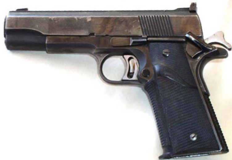
BEFORE — Showing extreme holster wear
